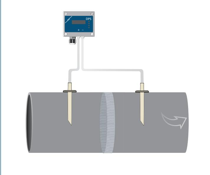
**Application 2:** Measuring supplied volume flow [m<sup>3</sup>/h] or air velocity [m/s] using PSET-PT Pitot tube connection set
