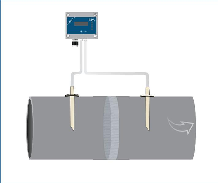
**Application 2:** Measuring volume flow [m<sup>3</sup>/h] or air velocity [m/s] using PSET-PT
