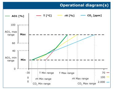
**Note:** The output changes automatically depending on the highest of the T, rH or  $CO_2$  values, i.e. the highest of the three output values controls the output. See the green line in the operational diagram above. One or multiple sensors can be deactivated. E.g. it is also possible to control the output based on the measured  $CO_2$  values only.
