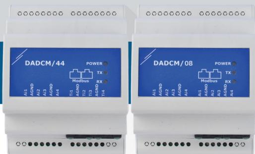
DADCM are DIN rail mounted analog to digital (Modbus RTU) converter modules supplied via Power over Modbus. The DADCM/08 product version has four analog / modulating and four analogue inputs while the DADCM/44 version has four analog / modulating inputs and four temperature inputs. The type of input is selected via Modbus RTU communication. The input values are transferred to Modbus RTU.
