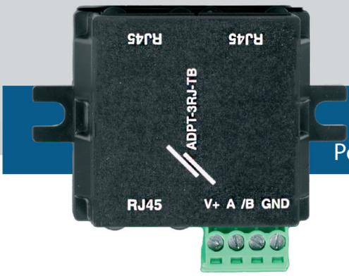
ADPT-3RJ-TB is an adapter for Power over Modbus (PoM) connection between three standard UTP network (RJ45) and one 4-pins terminal block. PoM is the Sentera standard for distribution of Modbus RTU (RS485) and power supply via a single RJ45 connector. The ADPT-3RJ-TB adaptor facilitates interconnecting Sentera devices with PoM to devices with regular terminal blocks.
